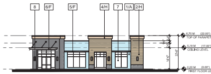
3 BUILDING 5 - SOUTH ELEVATION A-206 1/8" = 1'-0"
