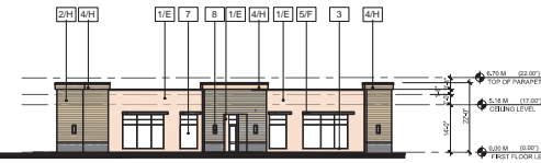
4 BUILDING 6 - EAST ELEVATION A-206 1/8" = 1'-0"
