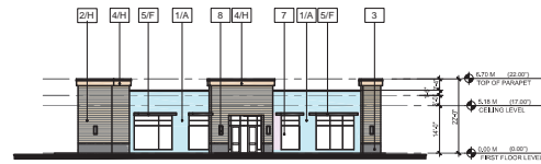
2 BUILDING 5 - WEST ELEVATION A-206 1/8" = 1'-0"
