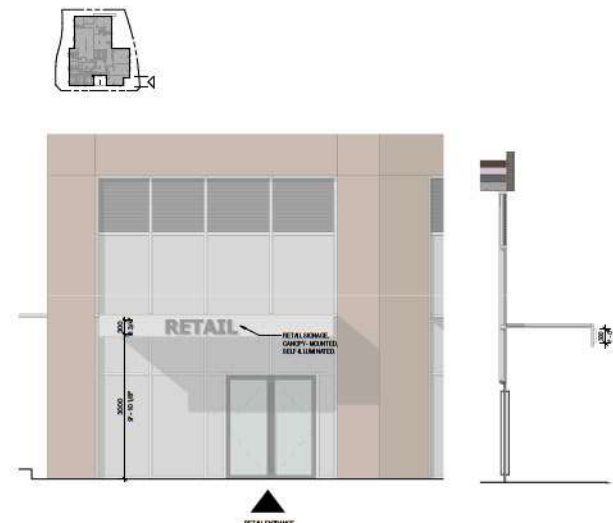
ELEVATION - SIGNAGE - EAST RETAIL ENTRANCE scale: 1:40
