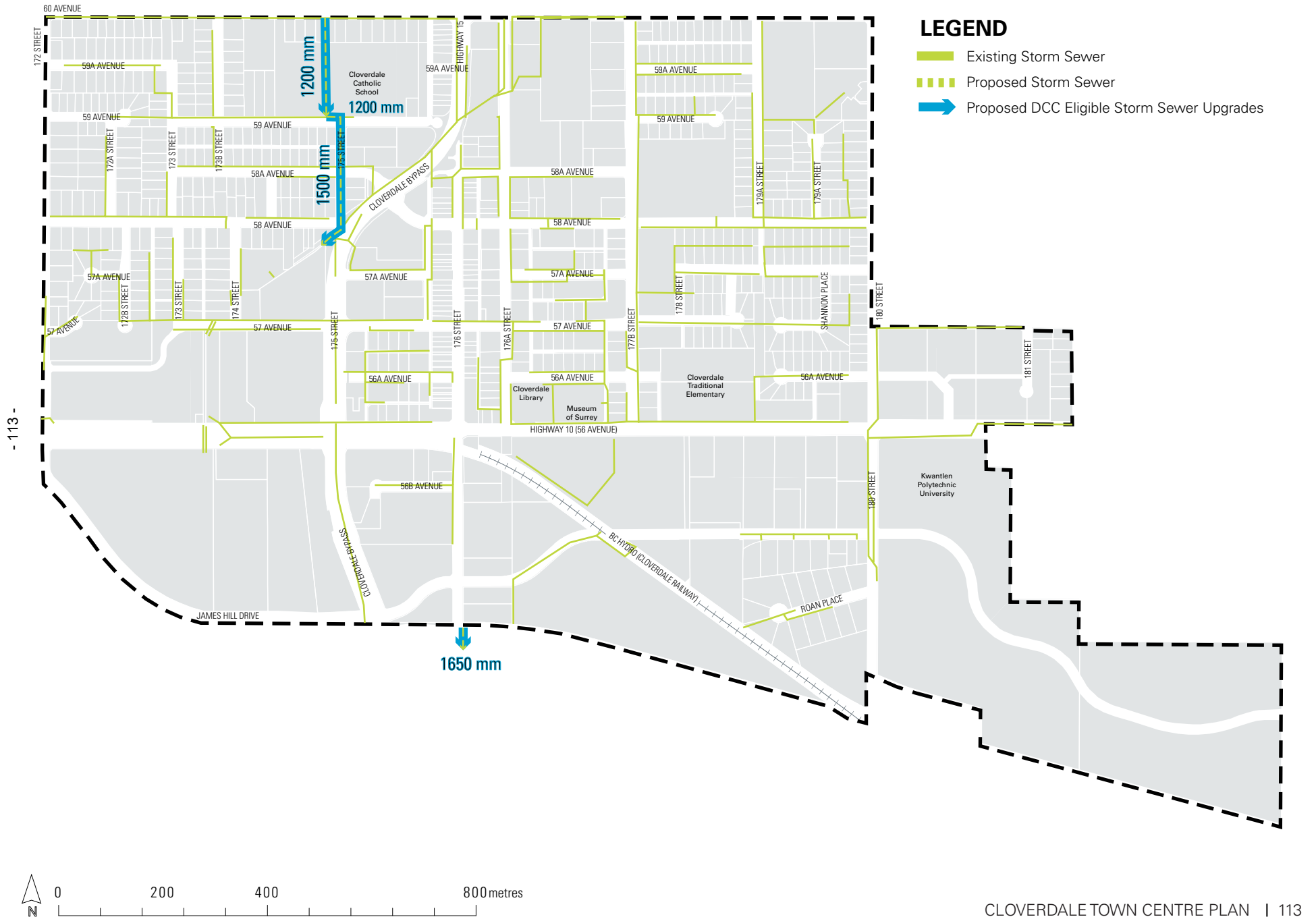
Figure 7.2: Drainage System Upgrades
