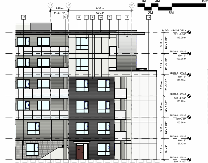
2 BUILDING 1 - SOUTH-EAST ELEVATION
