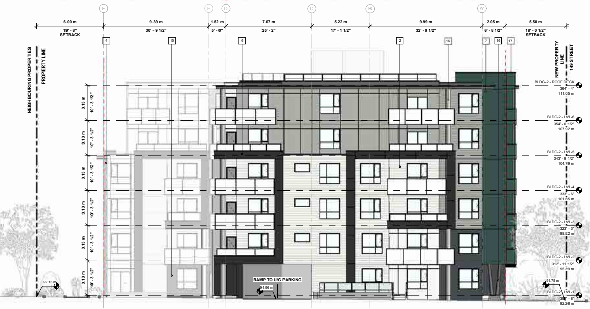
2 BUILDING 2 - NORTH ELEVATION [91A AVENUE] A-303 1/8" = 1'-0"
