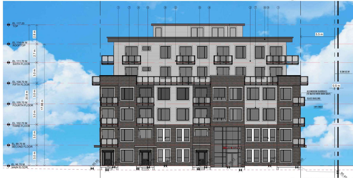
2 EAST ELEVATION (ALONG 149 STREET) Scale: 1/8"=1'-0"
