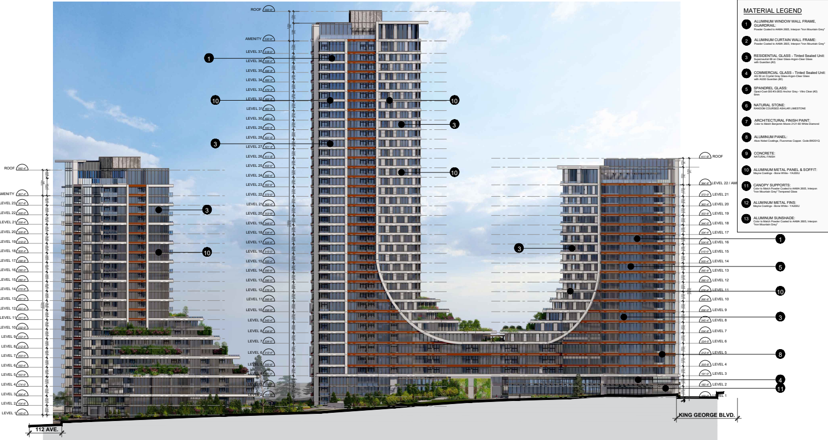
EAST ELEVATION OVERALL BUILDING ELEVATIONS SUBMISSION TO COUNCIL January 29, 2024
