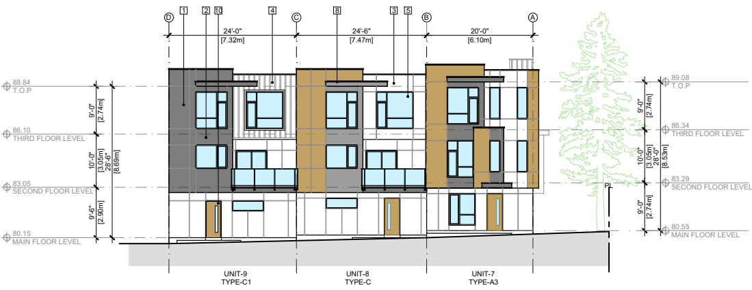
3 BUILDING-2 WEST ELEVATION Scale: 1/16" = 1'-0"
