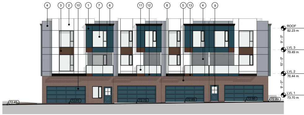
1 BLDG-1 NORTHEAST ELEVATION SCALE: 1/16" = 1'-0"
