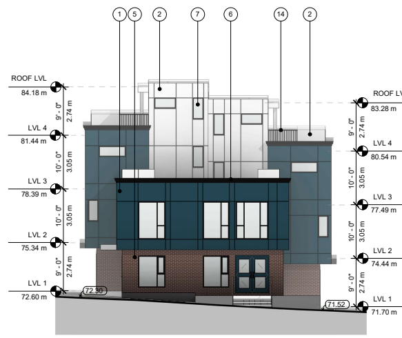
4 BLDG-2 SOUTHEAST ELEVATION SCALE: 1/16" = 1'-0"
