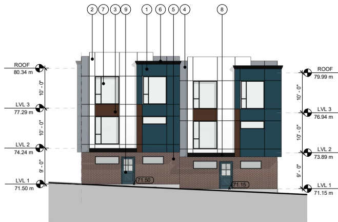
4 BLDG-4 SOUTHEAST ELEVATION SCALE: 1/16" = 1'-0"
