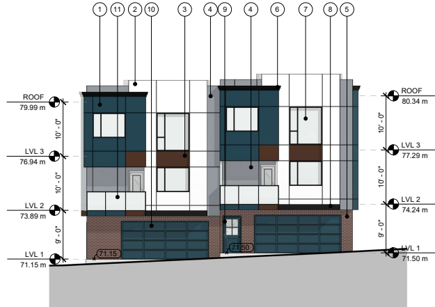
2 BLDG-4 NORTHWEST ELEVATION SCALE: 1/16" = 1'-0"
