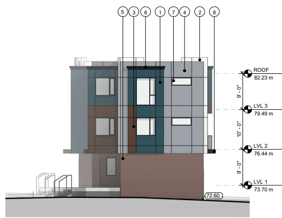
4 BLDG-1 SOUTHEAST ELEVATION SCALE: 1/16" = 1'-0"
