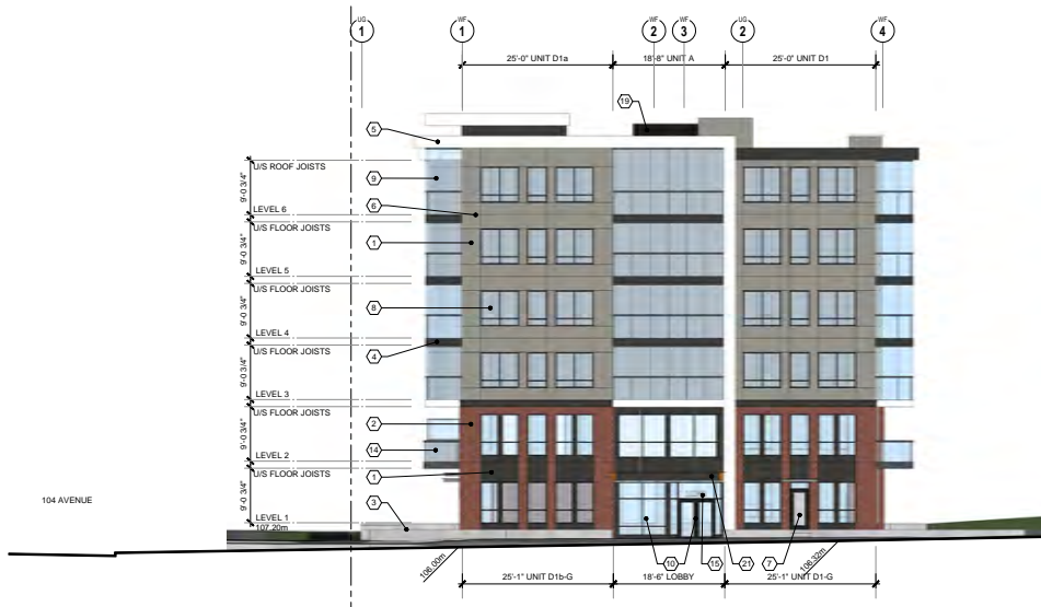
EAST ELEVATION (147 STREET) SCALE: 3/32" = 1'-0"
