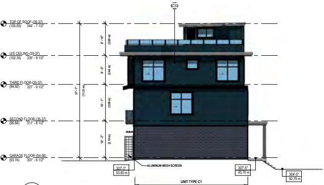
4 WEST ELEVATION DP-6.81 1/8" = 1'-0"
