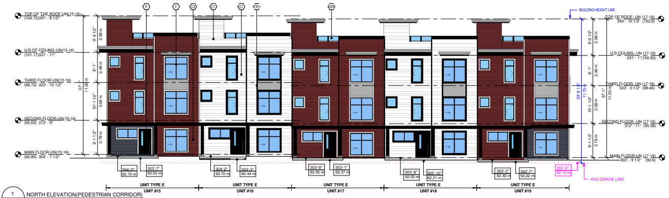
1 NORTH ELEVATION/PEDESTRIAN CORRIDOR DP-6.51 1/8" = 1'-0"
