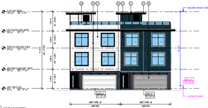
1 SOUTH ELEVATION DP-6.191 1/8" = 1'-0"
