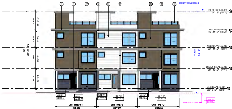
1 NORTH ELEVATION (PEDESTRIAN CORRIDOR) DP-6.31 1/8" = 1'-0"
