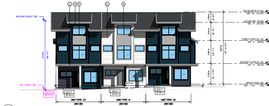
1 EAST ELEVATION (167 ST) DP-6.11 1/8" = 1'-0"
