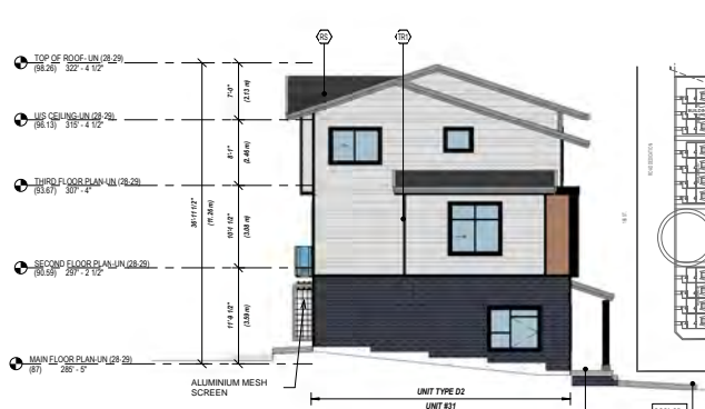
4 WEST ELEVATION DP-6.91 1/8" = 1'-0"
