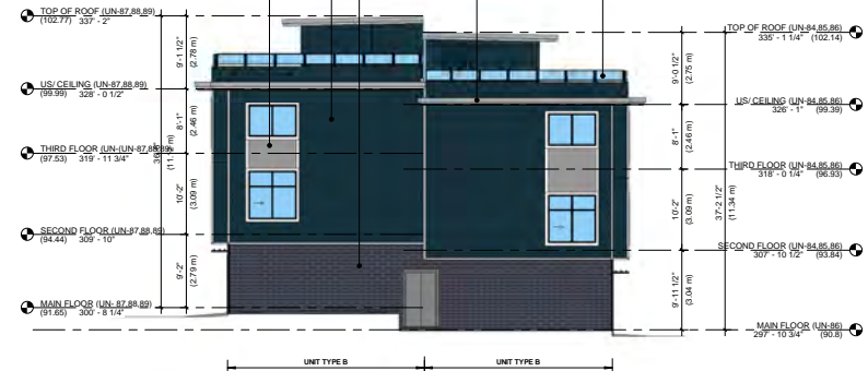
4 WEST ELEVATION DP-6.231 1/8" = 1'-0"
