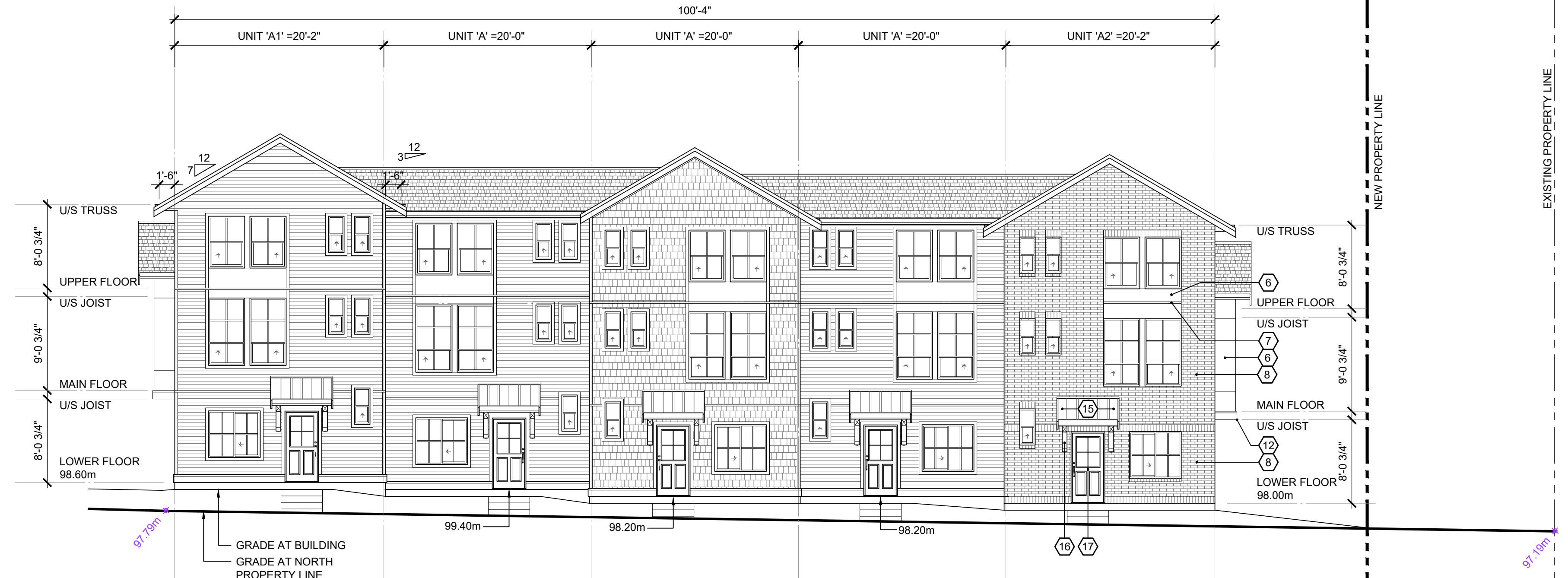
FRONT ELEVATION AT 25 AVENUE (NORTH) SCALE: 1/8"=1'-0"
