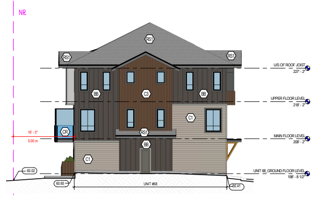
4 BUILDING-13 SOUTH ELEVATION SCALE: 1/8" = 1'-0"
