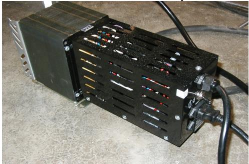
Ballast For Either High Pressure Sodium Or Metal Halide Lamp
