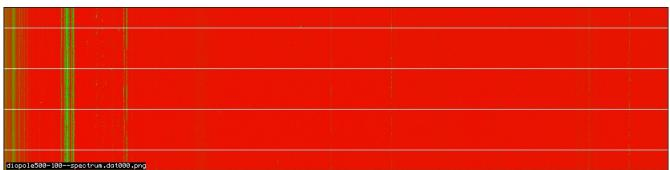
In this series of spectrum scans and a composite spectrogram, we see some signals in the HF region under 50MHz in the first division and some FM broadcast stations around 100MHz at the first division. There are no obvious signals generated by the HPS or MH lamps.
