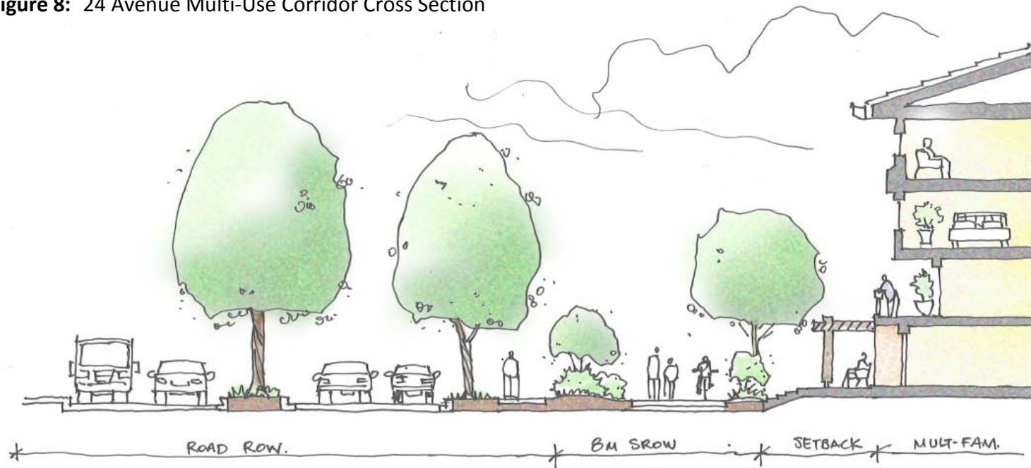
Figure 8: 24 Avenue Multi-Use Corridor Cross Section
