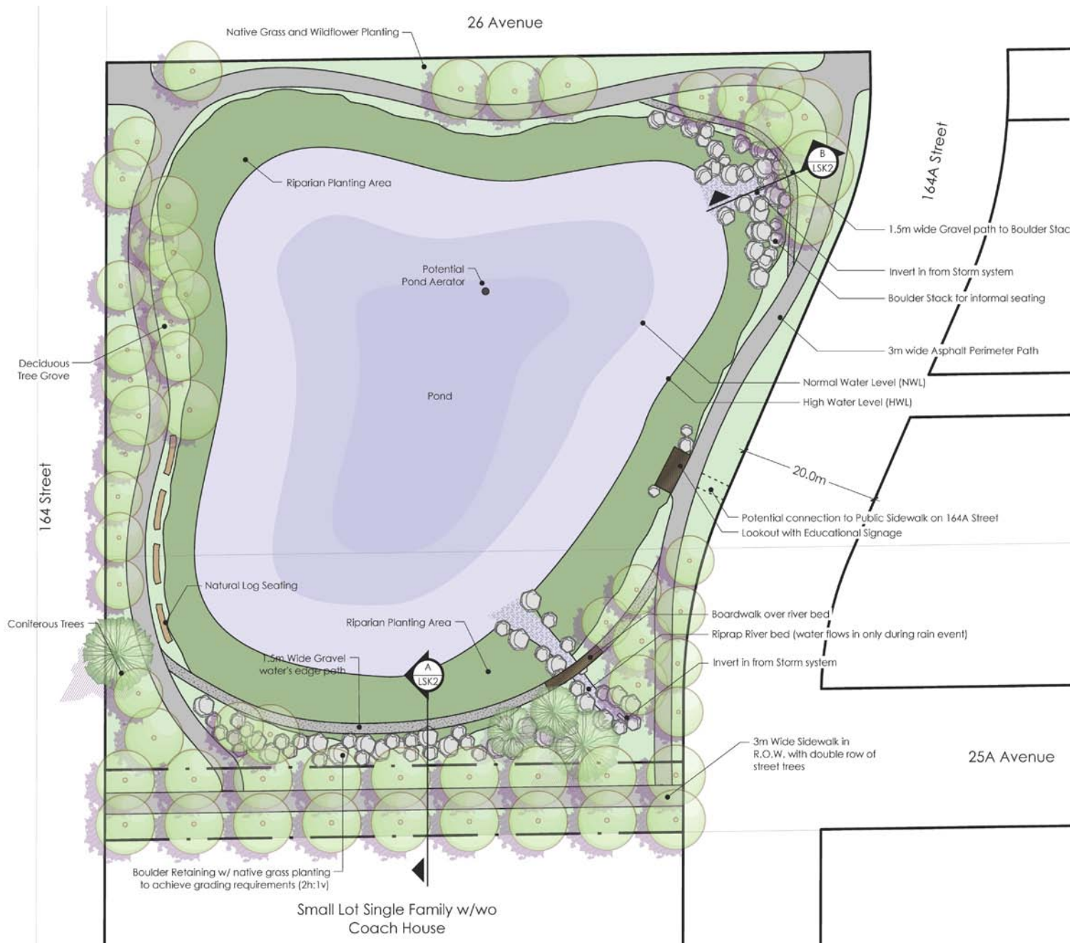
Figure 11: Stormwater Detention Pond Designed as a Community Amenity
