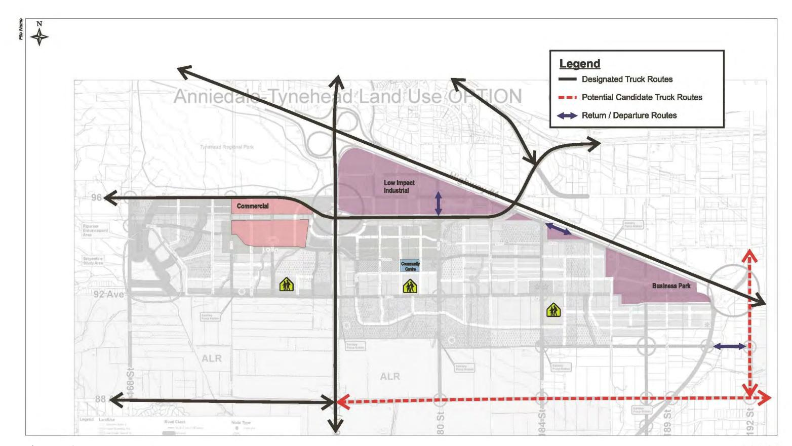
Figure 5.13 Preliminary Truck Route Plan
