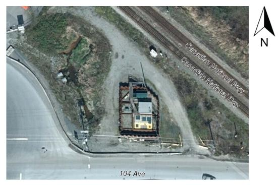
The pump station is located at 3 metre geodetic ground elevation. This is within the 200-year floodplain of the Fraser River, which makes it susceptible to flooding during extreme freshet events and a challenge to access and operate. The City has installed temporary flood protection works at the pump station site and has begun developing plans for the relocation and upgrade of the Big Bend Pump Station to ensure its long term operation.
