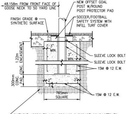
SUITABLE APPROVED NON-ORGANIC SUBGRADE COMPACTED TO 95% MPD. EXCAVATION OF ORGANIC/UNSUITABLE MATERIAL & BACKFILLING WITH IMPORTED GRANULAR FILL OR APPROVED NON-ORGANIC EXCAVATED MATERIAL WILL BE REQUIRED. (REFER TO GEOTECHNICAL REPORT FOR DETAILS)
