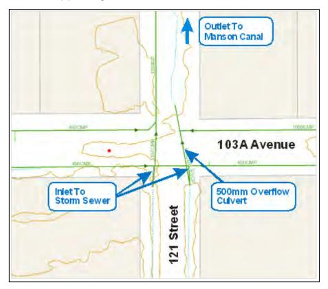
Figure 4.3 - Conveyance Piping at Intersection of 121 St and 103A Avenue
