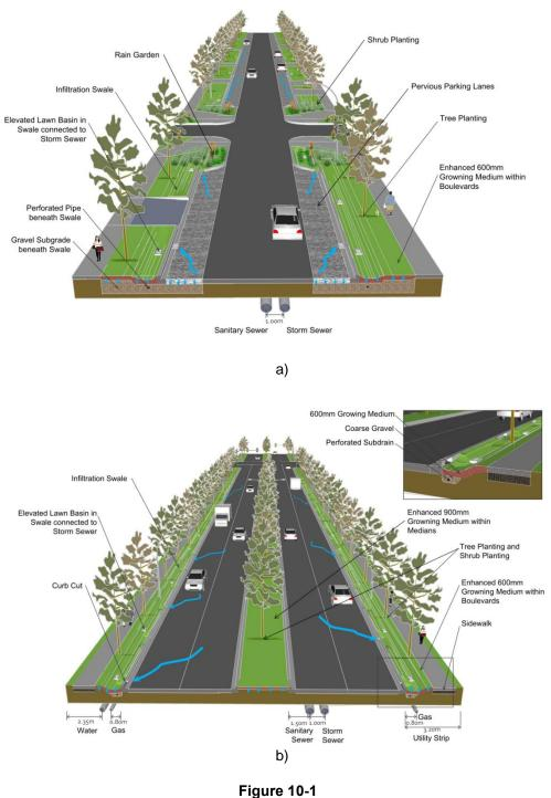
Road Right-of-Way Source Control / BMP Configurations a) Local and Collector Roads
