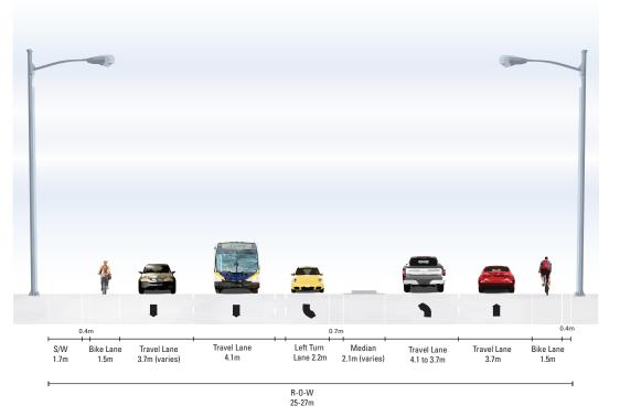
Figure 4.3: Highway 15 Typical Section, Curb and Gutter Raised Median
