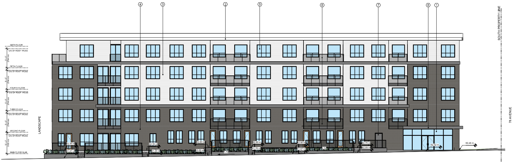
① LOT 2 BUILDING 3 - WEST ELEVATION 1/8" = 1'-0"
