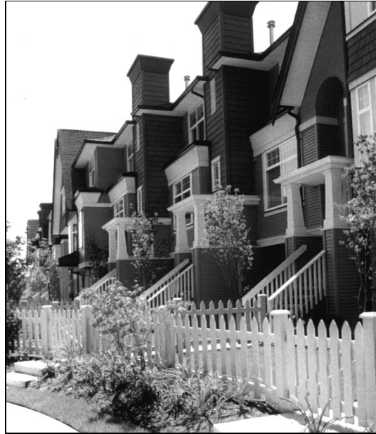
On this row-house street, all units access the street from a recessed front entry and a small front porch. Low fences (1 metre/3.3 feet) and landscaping distinguish public from private space and contribute to a neighbourly character.
