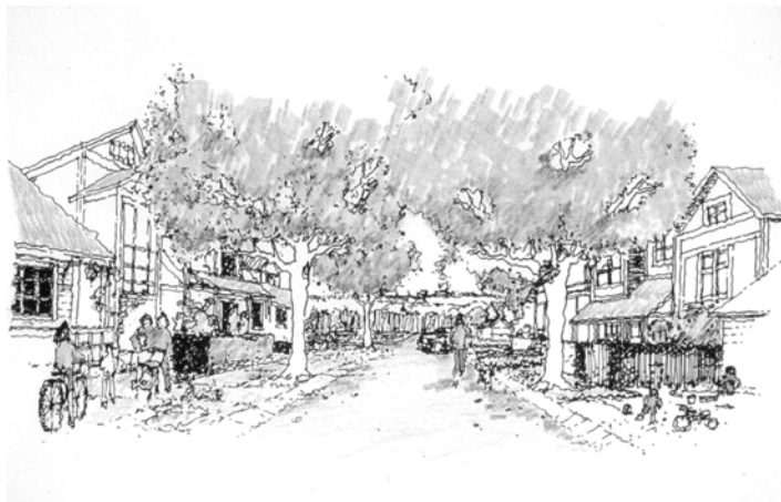
This image shows the ultimate desirable narrow, curbless residential street. Its curbless profile would allow water to infiltrate directly into the infiltration zone.
