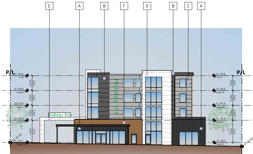
2 SOUTH ELEVATION ( KING GEORGE HIGHWAY ) 1/24"=1'-0"
