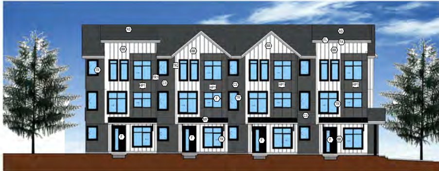
2 COLORED EAST ELEVATION DP-6.51 1/8" = 1'-0"
