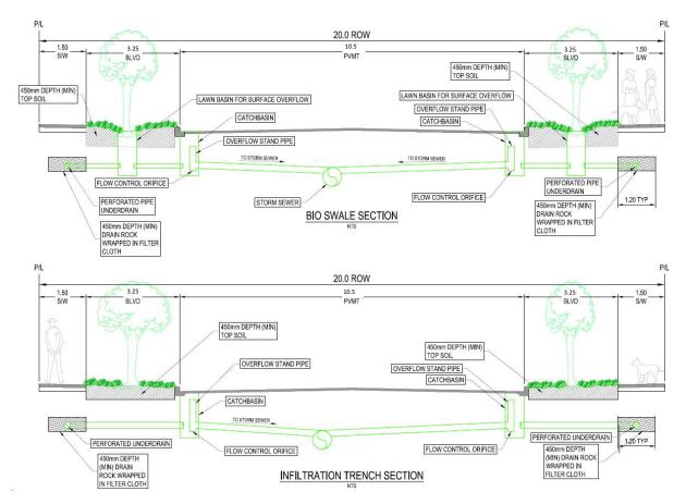
Figure 6.3 20 M Road Right-of-Way Bioswale & Infiltration Trench Cross-sections
