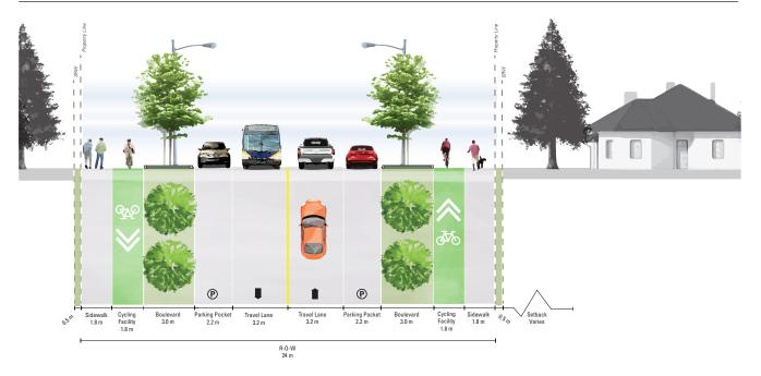
Figure 4.6 Standard Collector Road 24 m Cross-section
