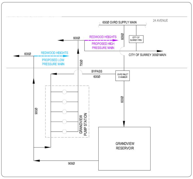
Figure 6.14 Proposed Feeder Main Connections
