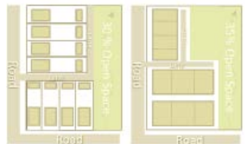
Example of 30-35% open space provided on a 1 acre Medium Density Cluster lot at 8 and 10 UPA.
