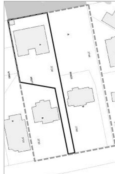
An example of a typical suburban panhandle lot with limited road access available, adjacent to an encumbrance.
