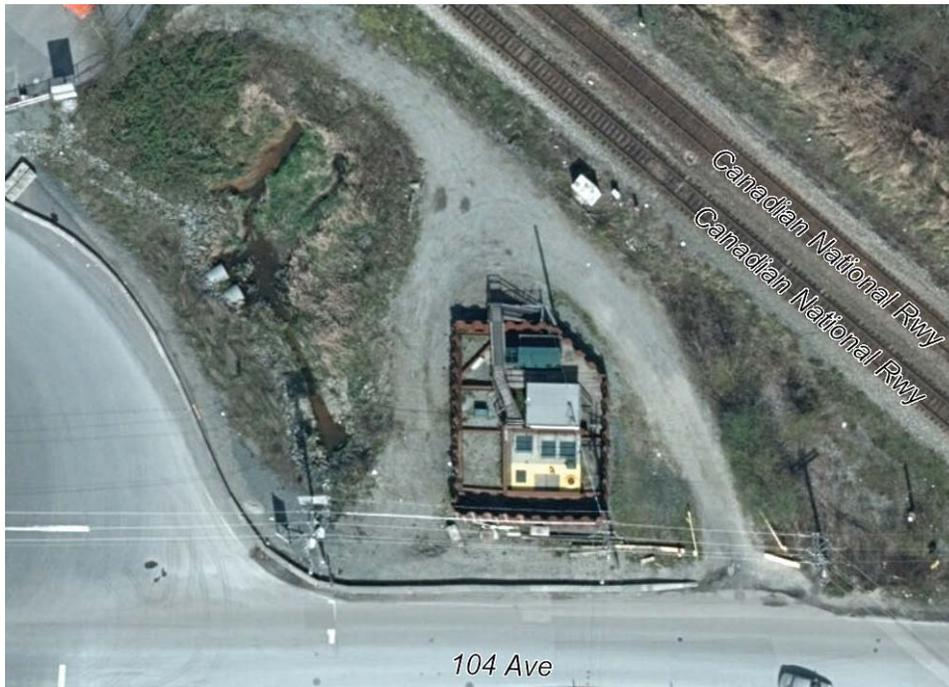
The pump station is located at 3 metre geodetic ground elevation. This is within the 200-year floodplain of the Fraser River, which makes it susceptible to flooding during extreme freshet events and a challenge to access and operate. The City has installed temporary flood protection works at the pump station site and has begun developing plans for the relocation and upgrade of the Big Bend Pump Station to ensure its long term operation.
